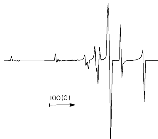
FIG. 2. Simulated spectrum of copper(II)-63 bis(morpholine- N -carbodithioate).
