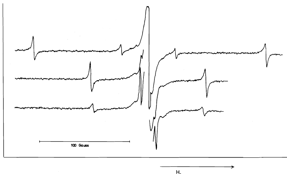
FIG. 1. Single crystal epr spectra of NMQ-TCNQ at 230 K. Spectra of three different crystal orientations (rotation of the crystal around an axis perpendicular to the field direction) which show the angular dependence of the triplet exciton splittings are drawn. The central peak corresponds to the 'impurity' peak.
