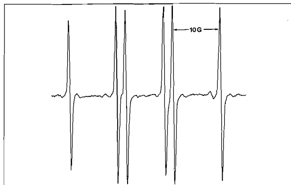
FIG. 2. The esr spectrum of the \cdot\text{CO}_2^- adduct of DMPO generated by \text{TiCl}_3 and \text{H}_2\text{O}_2 .
