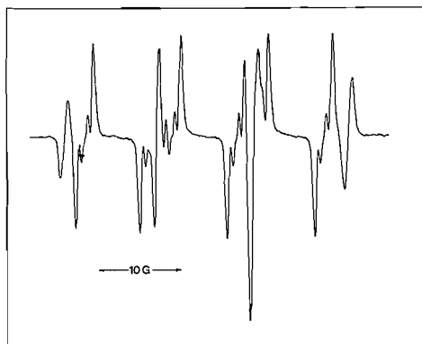
FIG. 1. The esr spectrum resulting from photolysis of an aqueous \text{Na}_2\text{S}_2\text{O}_8 ( 3 \times 10^{-3} M ) solution containing DMPO ( \sim 1 M ). The \cdot\text{OH} adduct (1:2:2:1) is superimposed upon the \text{SO}_4^{\cdot-} spectrum (see text).
